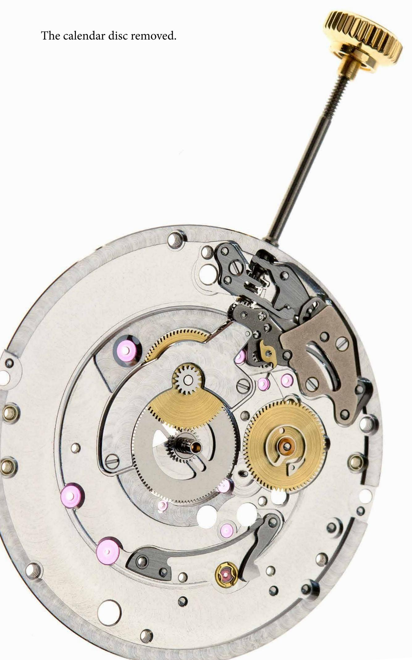
To the left the setting mechanism with three positions, neutral for winding, first position out, is for the rapid date change and the second postion to set the time.
